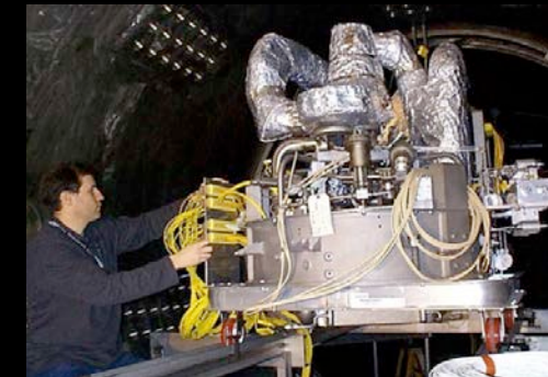
2kW Mini-BRU power conversion unit
